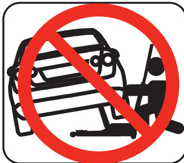
This hydraulic trolley jack should be used for lifting and lowering only; The raised vehicle should be supported on two vehicle support stands.
